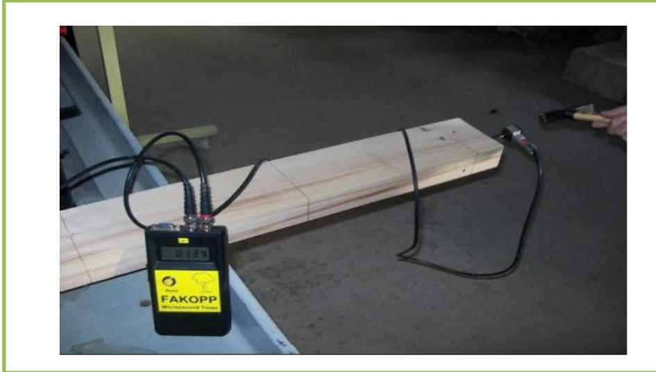
**Figura 13: Medidor Fakopp Microsecond Timerel**
