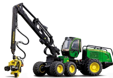
Figura 3.2 Maquina forestal harvester
