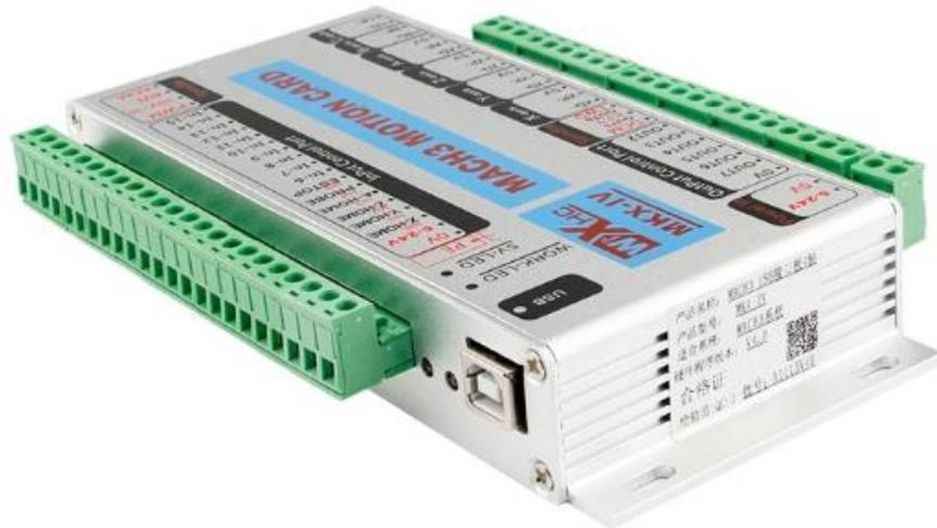
Fig. 66 Controlador CNC Wi-XHC MKX-IV
