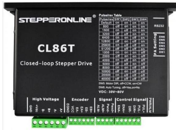
Fig. 53 Closed-loop stepper driver de STEPPERONLONE
