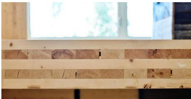
**Figura 2: Panel de CLT 5 capas (Souza, 2018).**
