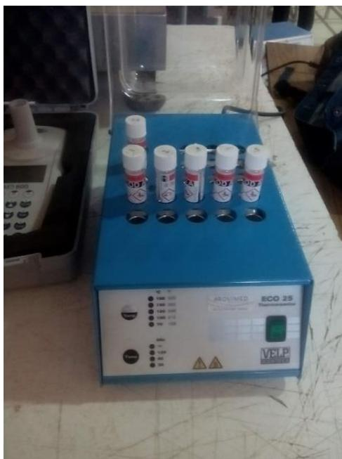
*Figura 24: Reactor Térmico “Velp Scientifica”.*
