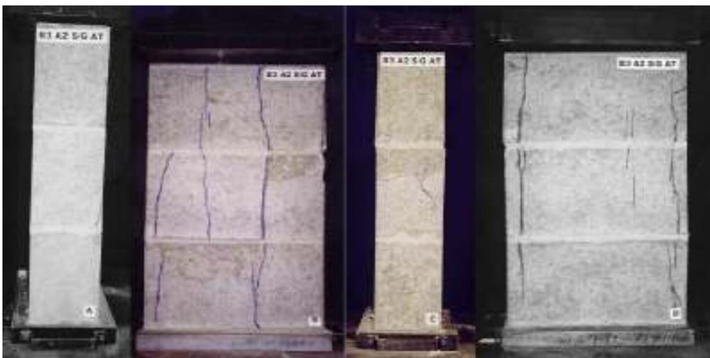
Figura 6.34 Modo ruptura prisma B3-A2-S/G-AT.
