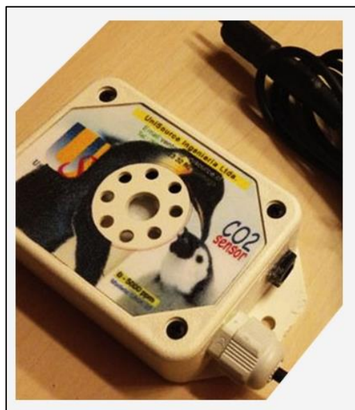
Figura B.1.2 Sensor CO 2 Unisource
