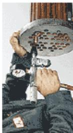
6. Release compressed air to the VLD by depressing the VLD lever trigger. The tube under test will evacuate rapidly for a few seconds, as registered by the vacuum gage (Key 17) and at a slower rate as the vacuum continues to build up.
